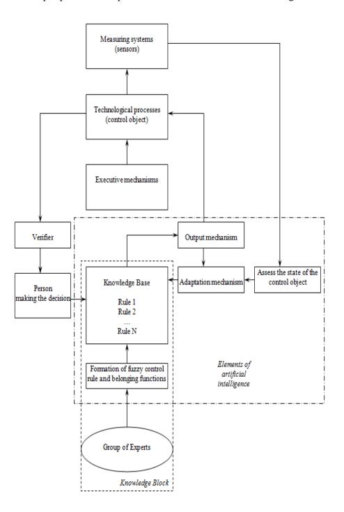
Figure 1 - Structure of the synergistic control system of multi-mode objects with neuro-fuzzy adaptation.
